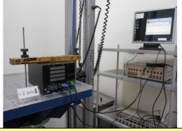
10. Mechanical Shock Test: +Z axis
