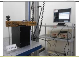
Mechanical Shock Test: +Y axis
