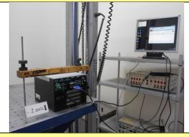
Mechanical Shock Test: -Z axis
