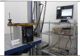
Mechanical Shock Test: -X axis
